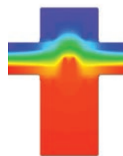
Thermal cross section: Less heat loss indicated by the red colour
